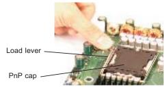
2. Gently lift the load lever to open the load plate.
